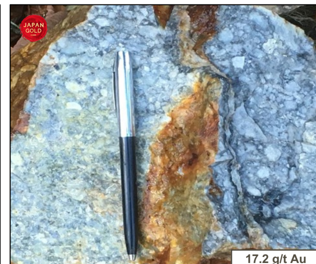
Sakinzawa Workings sample: gold-bearing quartz stockwork in rhyolitic breccia outcrop; SAM02069: 17.2 g/t Au, 16 g/t Ag
